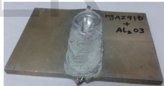
Fig.6: FSW Joint of AZ91 with Al 2 O 3
